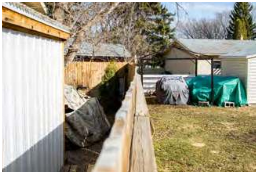
Photo: Ensure that sheds and items stored along the fence are a minimum 0.5 metres (20 inches) away.
