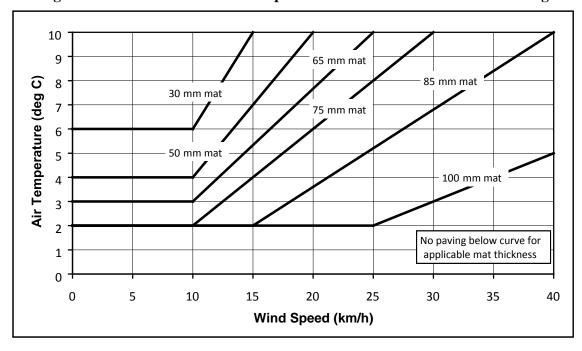
Figure 3.1 – Guidelines for Air Temperature and Wind Limitations on Paving
